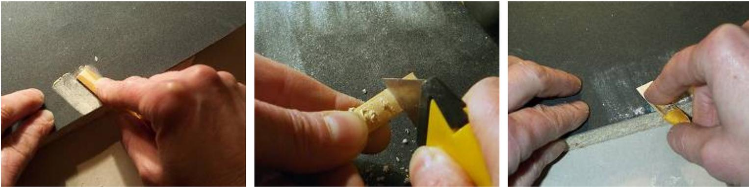
Once the reed blades start to flex and flatten to your satisfaction, (sorry, this is a case of trial and error, and practice), twist a piece of wire around the cane part just above the wrapping and secure the ends. This is the bridle. It can be used to make adjustments to the reed aperture. Use pliers over the bridle to gently squeeze the reed blades together. (I use two turns of tinned copper wire, 22 SWG, but some may prefer one or more turns of thinner or thicker wire).
