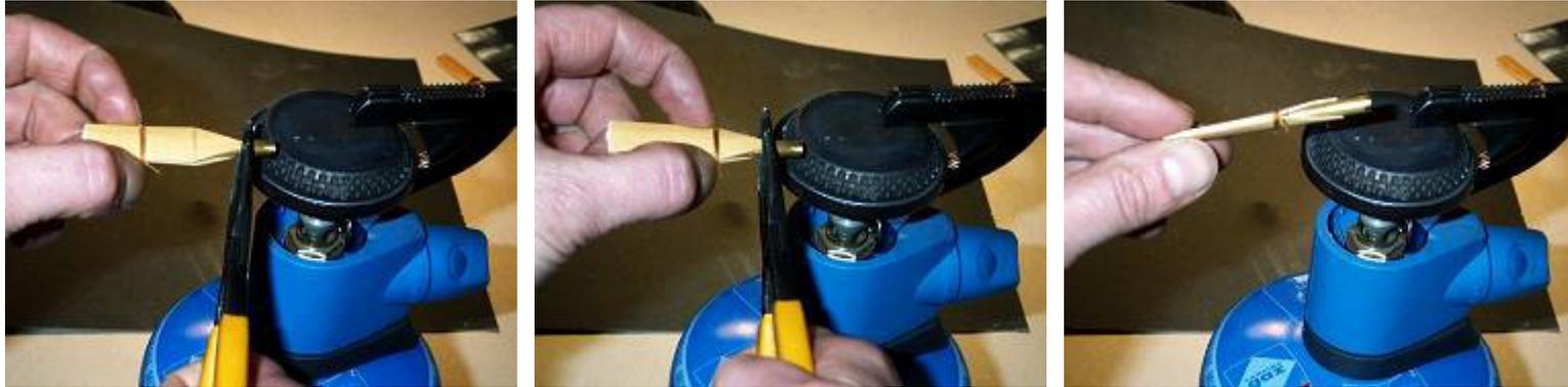
When cool, apply a small drop of superglue to each side of the points and allow to dry with the staple end pointed slightly downwards - glue must not enter the upper body of the reed.
