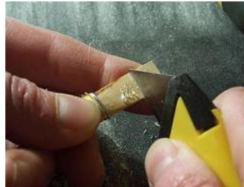
Open up the reed aperture a little by squeezing the sides of the bridge and check that the "lips" of the reed are not getting too thin. The reed will begin to "crow" when sucked (**blow the dust out first!**). Unlike Highland Bagpipe reeds, these reeds must not be exposed to moisture. Take great care not to over thin, especially the tip of the reed. Again, only trial and error and a lot of practice will tell you how to proceed at this stage.
