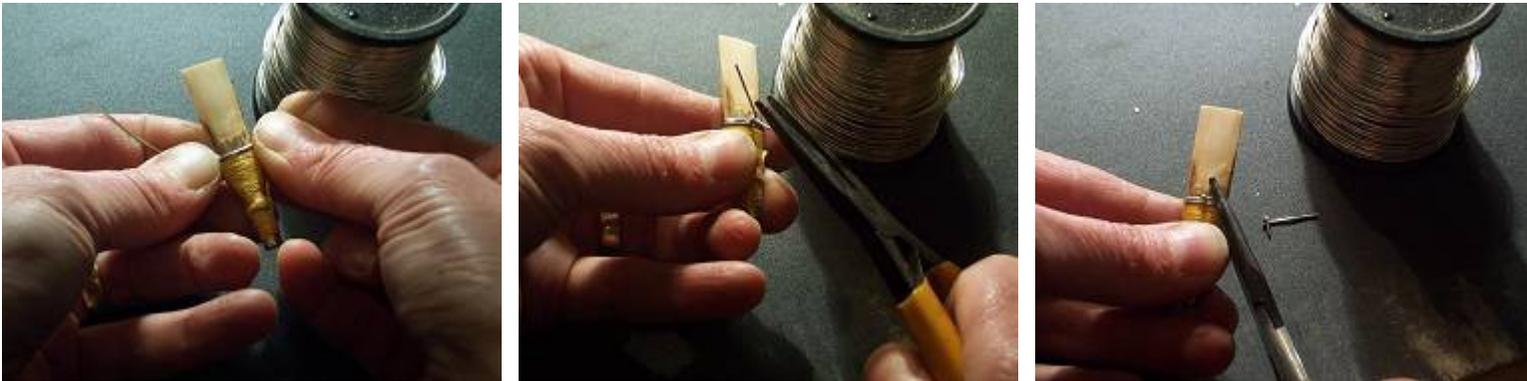
Continue with some gentle sanding (400 or 600 grit wet and dry) and scraping if necessary, then trim the end of the reed with a sharp blade, so that the total length of the reed is 51mm. Use the reflection in the knife again to ensure you are cutting squarely. I use a small cutting block for this job. Continue sanding and scraping, checking against the light.
